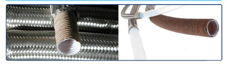
Inner core of virgin corrugated PTFE with PTFE impregnated fibre glass tape and a high tensile stainless steel 304 wire braid. Each corrugation has a low profile to promote easy cleaning.
