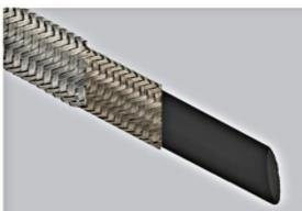
ABCOFLEX smooth bore is a quality engineered plain PTFE tube reinstated with double AISI 304 high tensile stainless steel braid. They are designed specifically for industrial use where reliability and long life are required and where hostile temperatures or corrosive conditions make PTFE the ideal choice. Abcoflex is available with translucent virgin PTFE or anti-static black.
