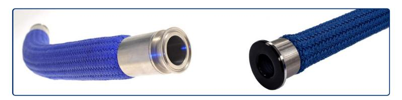
Polypropylene braided hose is often preferred in applications where aggressive environment tend to corrode SS braid. PP braid is lighter in weight and provides extreme flexibility. The tube is available in virgin or conductive black where electrostatic dissipation is required. Also available special vacuum resistant hose.
